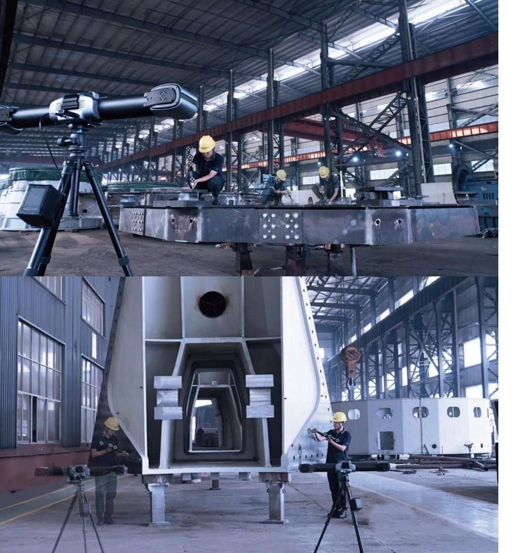
The probe locations can be approached from any angle as long as the i-Probe is within the optical tracker cameras' field of view. i-Probe's poses can be tracked and mapped to the coordinate systems in real time by the tracker so that it can measure continuously without the need to reposition.
